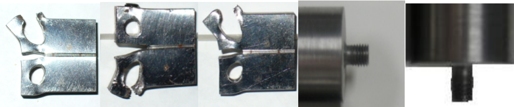
Figure 4. Deformed CT samples and the threaded grip part before and after deformation.
