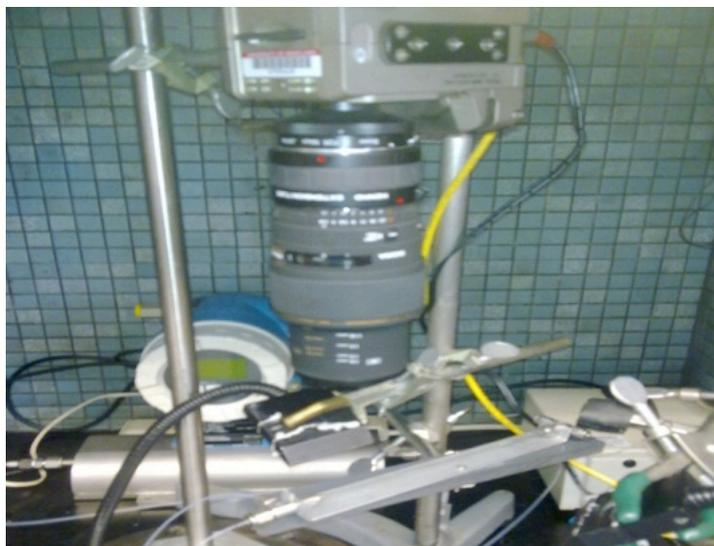
**Figure 12. Phantom MIRO - 4M high-speed camera.**
