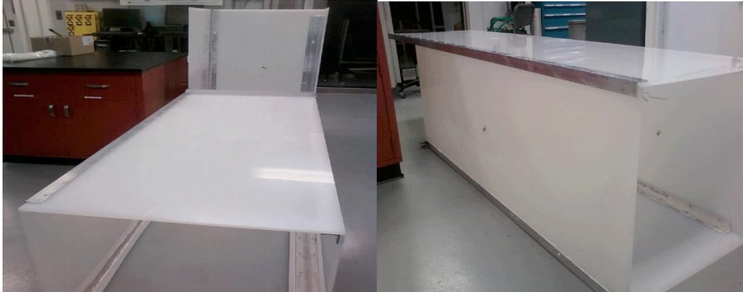
**Figure 5. The two ducts used to construct the conditioned space.**
