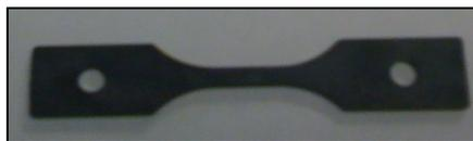
Figure 11. Carbon reinforced nylon tensile specimen.
