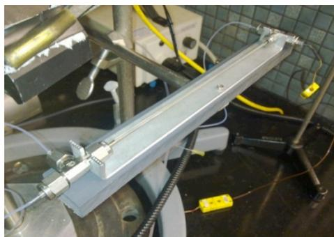
**Figure 9. Channel support in the microreactor.**
