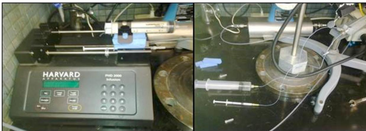
**Figure 11. Syringe pump with different diameter of syringes.**
